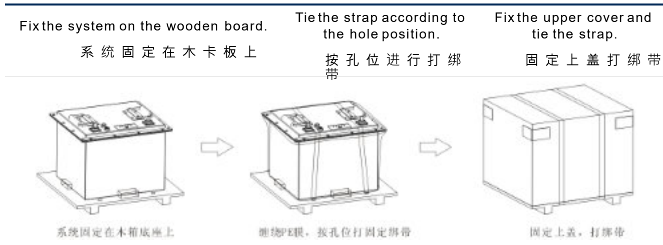
Figure 2. Schematic Diagram of Packaging
