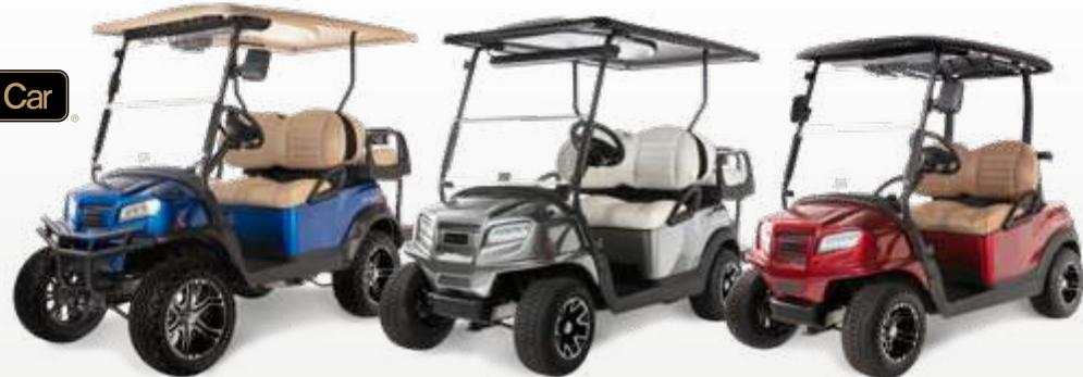
**Electric Onward PTVs** feature smart chargers that issue alerts to prevent common user errors. The vehicles are also available with optional on-board chargers and reel retractors that allow for opportunity charging at any 110-volt outlet. *(Images shown include optional upgrades.)*
